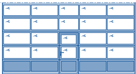
Sectional door ALR F42 with wicket door with trip-free threshold
