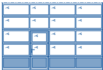
Sectional door ALR F42 with wicket door with trip-free threshold
