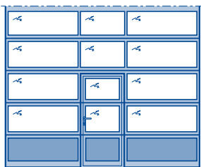
Sectional door ALR F42 with wicket door with trip-free threshold
